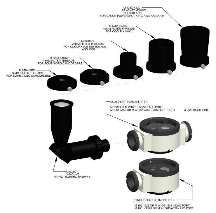
MOST CAMERAS REQUIRE THE X-MOUNT TO BE USED IN A 50/50 PORT
